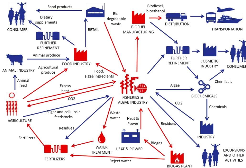
Figure 5. The business ecosystem of Sybimar. The parts of the aquatic biorefinery covered by Sybimar's solutions are presented in red color.
